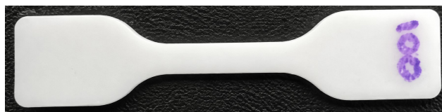
Fig. 5. Standard dumbbell-shaped adhesive specimen.
