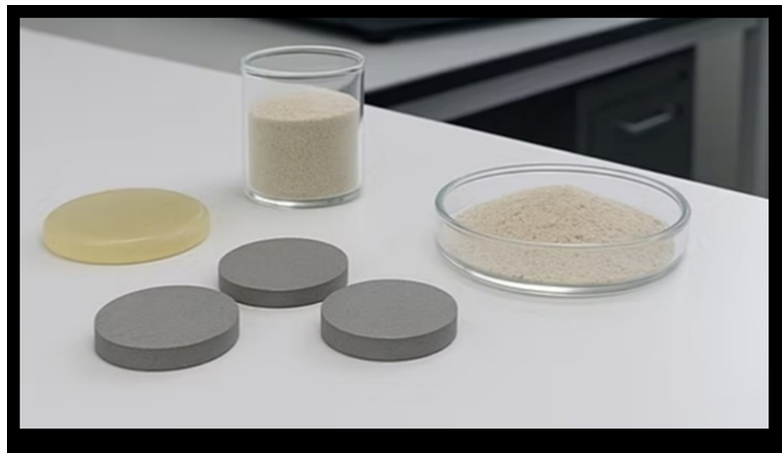
Fig. 4. Circular disc prepared from a stone sample.
