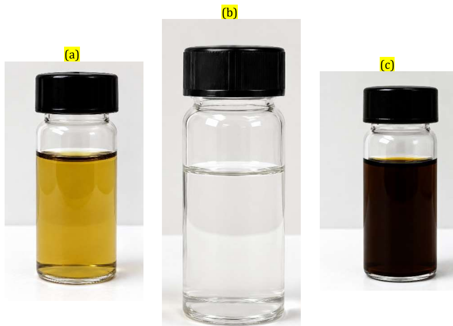
Fig. 2. Visual stages of AgNP synthesis: (a) aqueous leaf extract after filtration; (b) silver nitrate solution before reaction with plant extract; and (c) reaction mixture after the color change suggesting AgNP formation.
