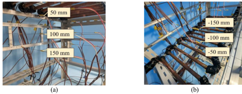
Figure 3. Measurement of air temperature vertically: areas (a) below and (b) above the heat exchanger.
