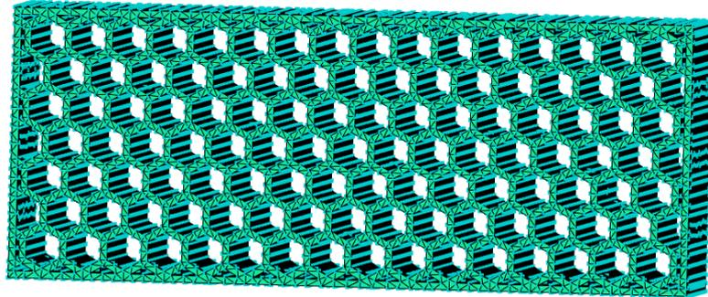
**Figure 2.** Mesh model of honeycomb brick
