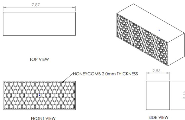
**Figure 1.** Geometry and specification of honeycomb brick
